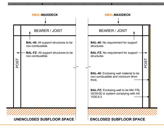
This diagram outlines the requirements under AS 3959-2009 Construction of buildings in bushfire-prone areas for the framing of verandas, decks, steps, ramps or landings for either BAL-40 or BAL-FZ construction.
